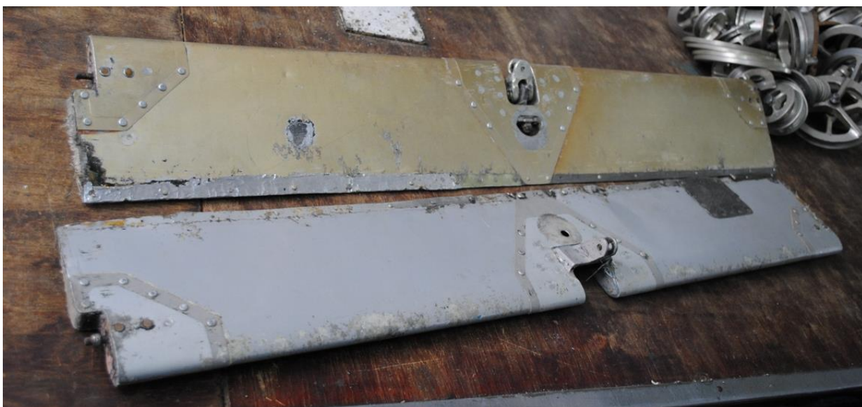
Corrosion of elevator trim tabs 32.02.3210.000.001 (002)
