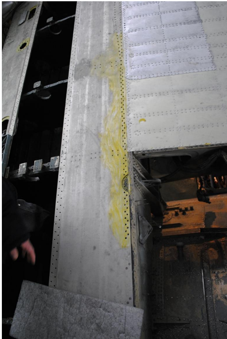
Center section corrosion (6 pads are installed)
