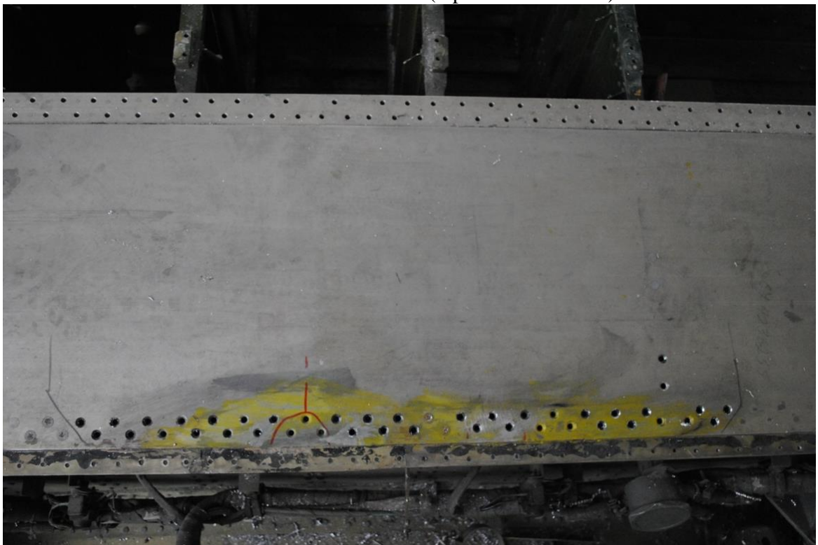
Center section corrosion (6 pads are installed)
