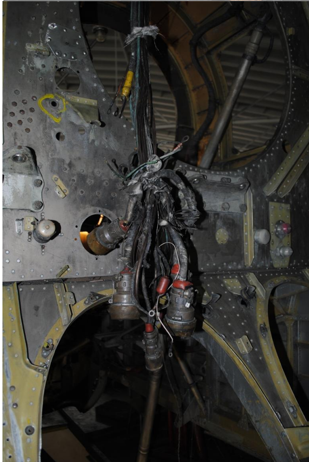
Right nacelle - wire breaks, corrosion of terminals, hinges
