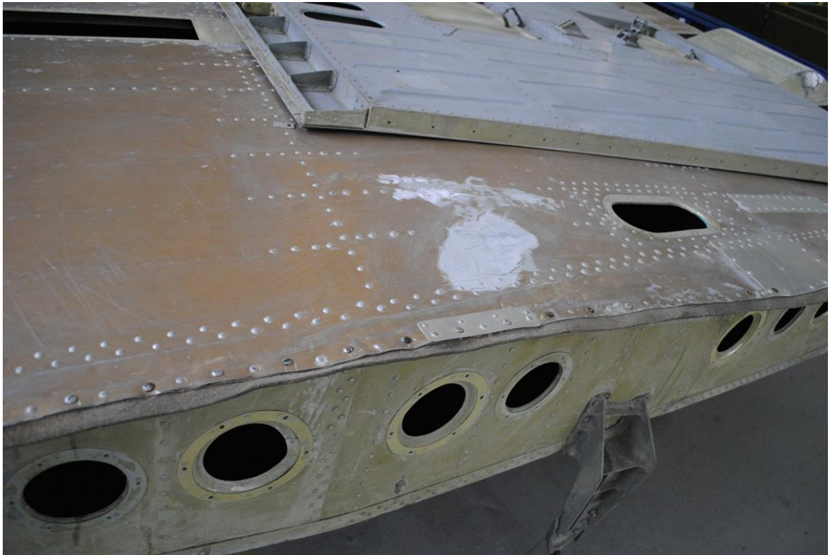
A ramp of another series has been installed in operation (it was 0209, now 0303).
