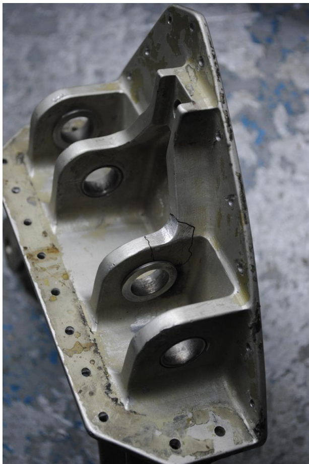
Slat bracket crack 32.02.3615.021.002
