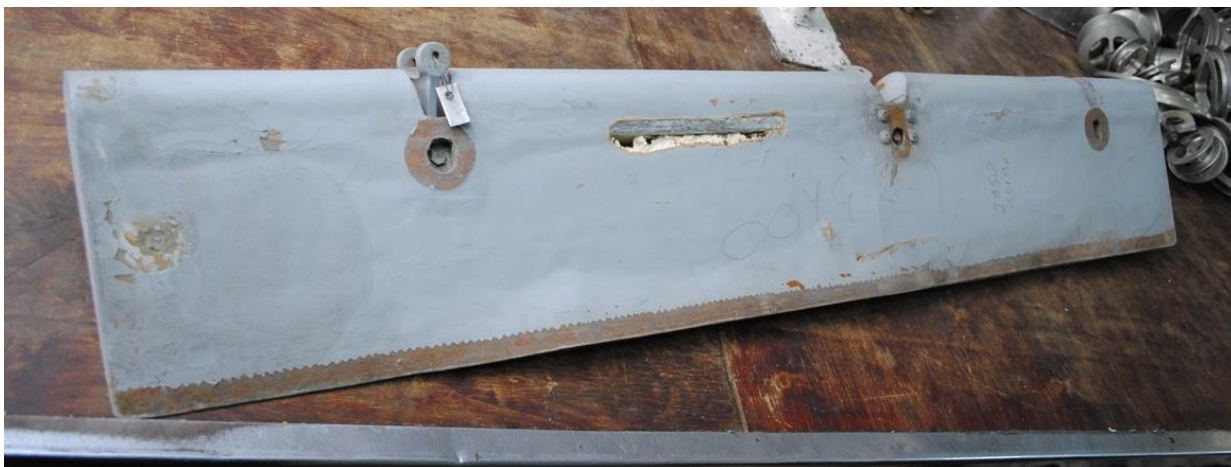
Corrosion and dents trim rudder trim 24-3707-0
