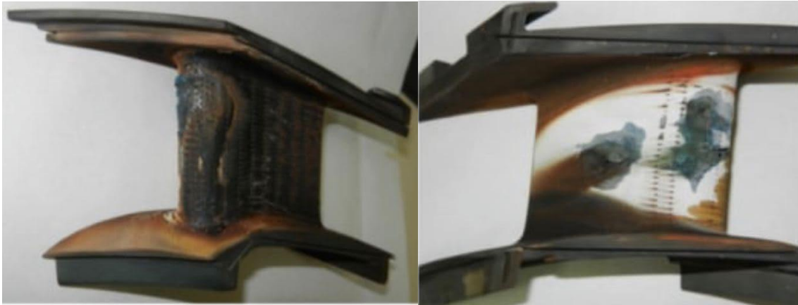
Figure 3.2 – Burnout of nozzle blades after testing
