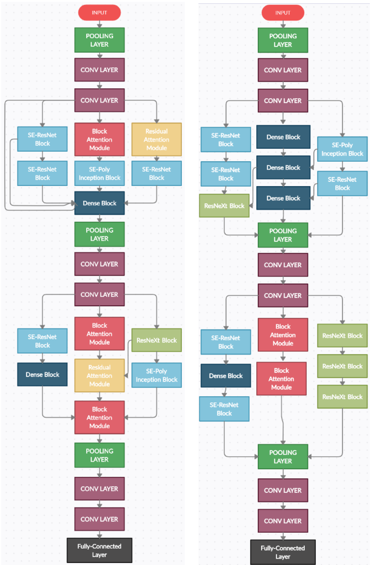
Fig. 3.4 Randomly generated CNN architectures using the genetic algorithm and special blocks
