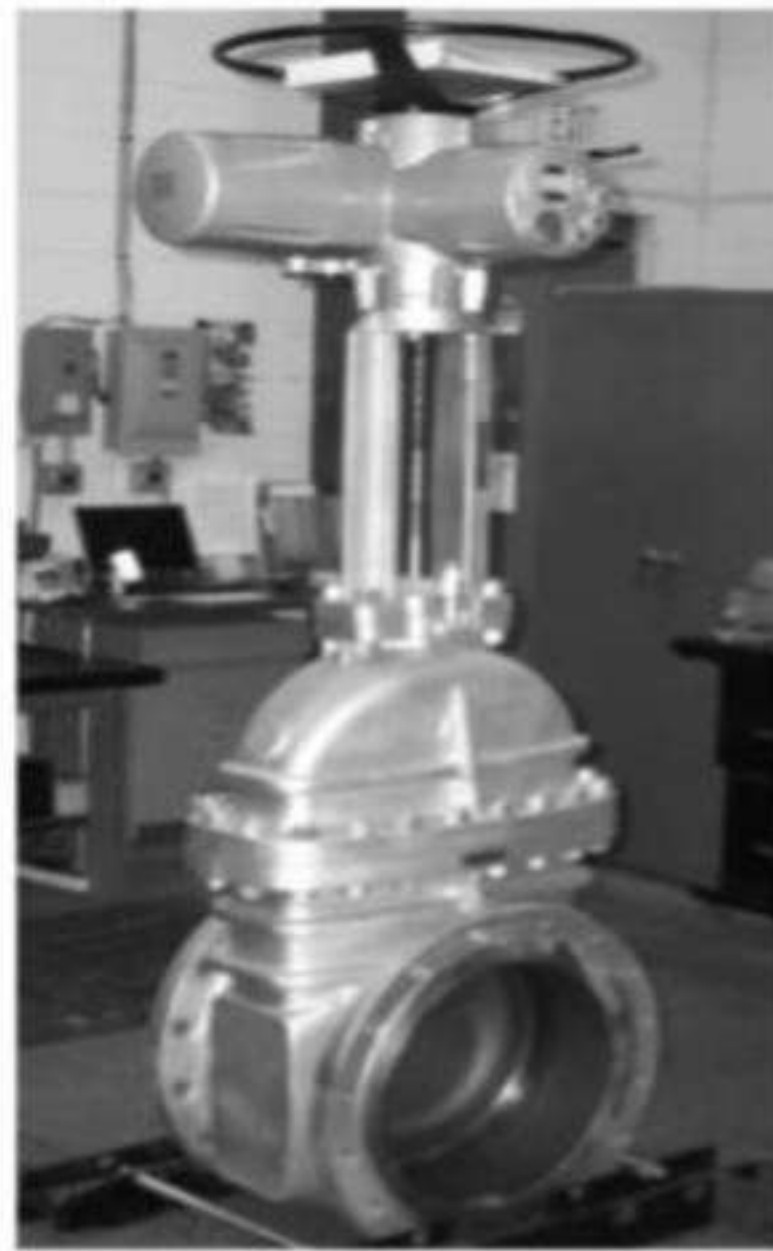
Figure 3.4 – BIFFI ICON 2000 electric actuator fitted onto a disassembled valve.
