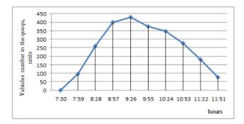
Fig. 4. The number of vehicles in the queue in front of the traffic light.
