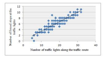
Fig. 1. The correlation field of the number of traffic lights along the traffic routes to the forced stops at them.
