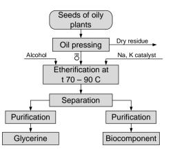
Fig. 5. Technological scheme of biocomponent production
