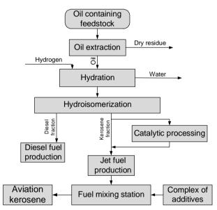
Fig. 6. Technological scheme of HVO kerosene production
