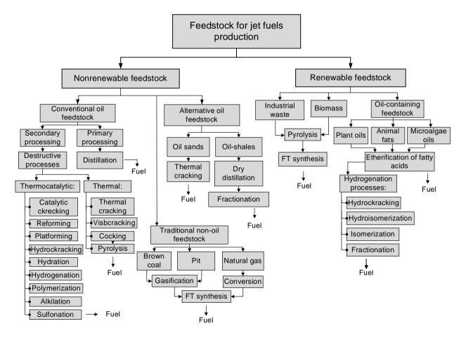
Fig. 1. Classification of technologies for jet fuel production according to the feedstock used [13-15]
