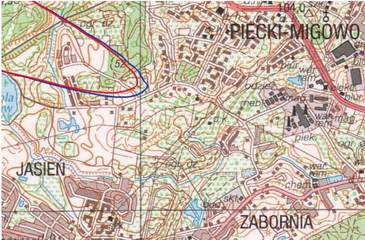
Figure 2. Comparison of the noise exposure contours for the two approach paths: blue-real profile, red- modified/CDA, L_{Aeq}=45\text{dB(A)} .
