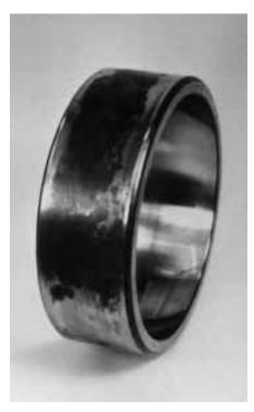
Figure 1.16–Fretting corrosion on the outer ring of a spherical roller bearing
