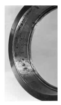
Figure 1.15 – Deep seated rust in the outer ring of a cylindrical roller bearing
