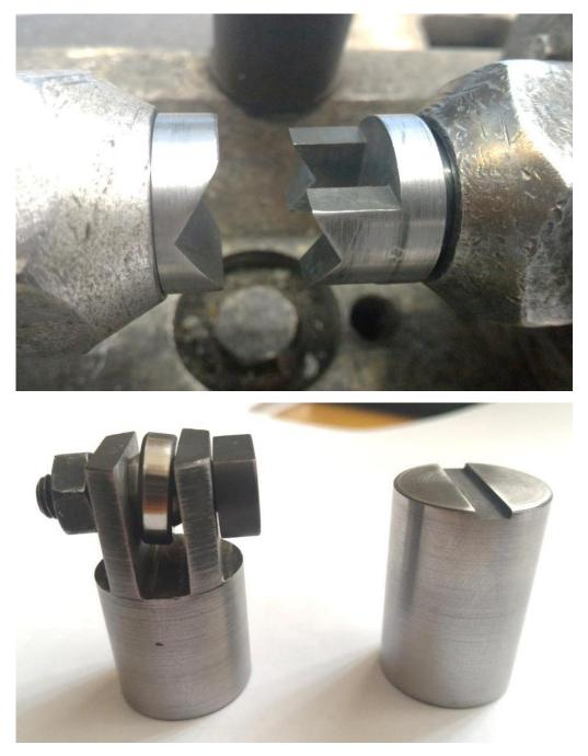
Figure - 3.5 Clips to hold the spherical plain bearings
