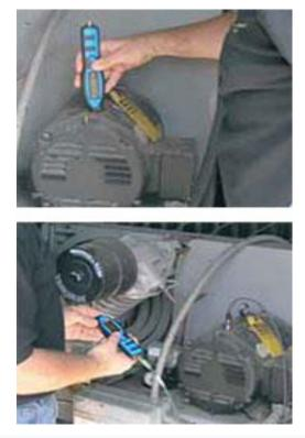
Figure 1.22 – Bearing vibration measurement
