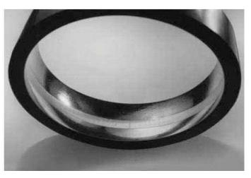
Figure 1.6 – Outer ring of a spherical roller bearing that has not been adequately lubricated. The raceways have a mirror finish
