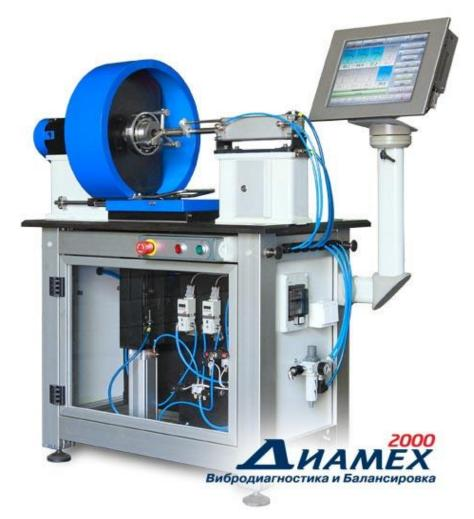
Figure 2.2– Stand of incoming inspection of bearings CΠ-180M (DIAMECH 2000)
