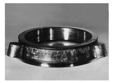
Figure 1.18– Flaked cone and rollers of taper roller bearing. Heavy loading and inadequate lubrication are the causes of this damage
