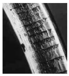
Figure 1.13 – Smeared face of a cylindrical roller bearing inner ring
