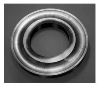
Figure 1.8 – Washer of a thrust ball bearing subjected to overloading while not running. The indentations are narrow and radially aligned, not sphered as in radial ball bearings
