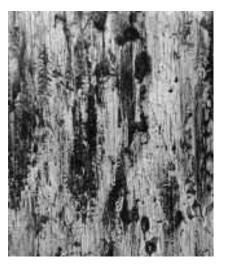
Figure 1.10 – Smearing on the surface of a roller from a spherical roller bearing –  $100 \times magnification$
