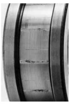
Figure 1.7 – Vibration damage to the ring of cylinder roller bearing.
