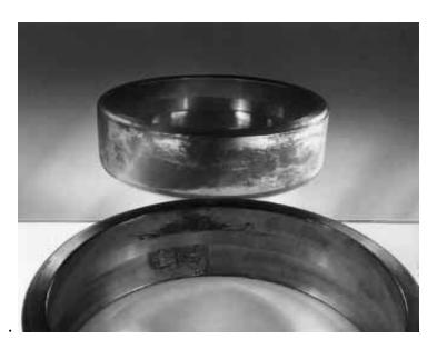
Figure 1.19 – Flaking in the raceways of the outer ring of a spherical roller bearing
