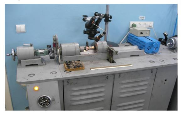
Figure - 3.1 Outward of settings M $\Phi$ K-1 testing at fretting corrosion
