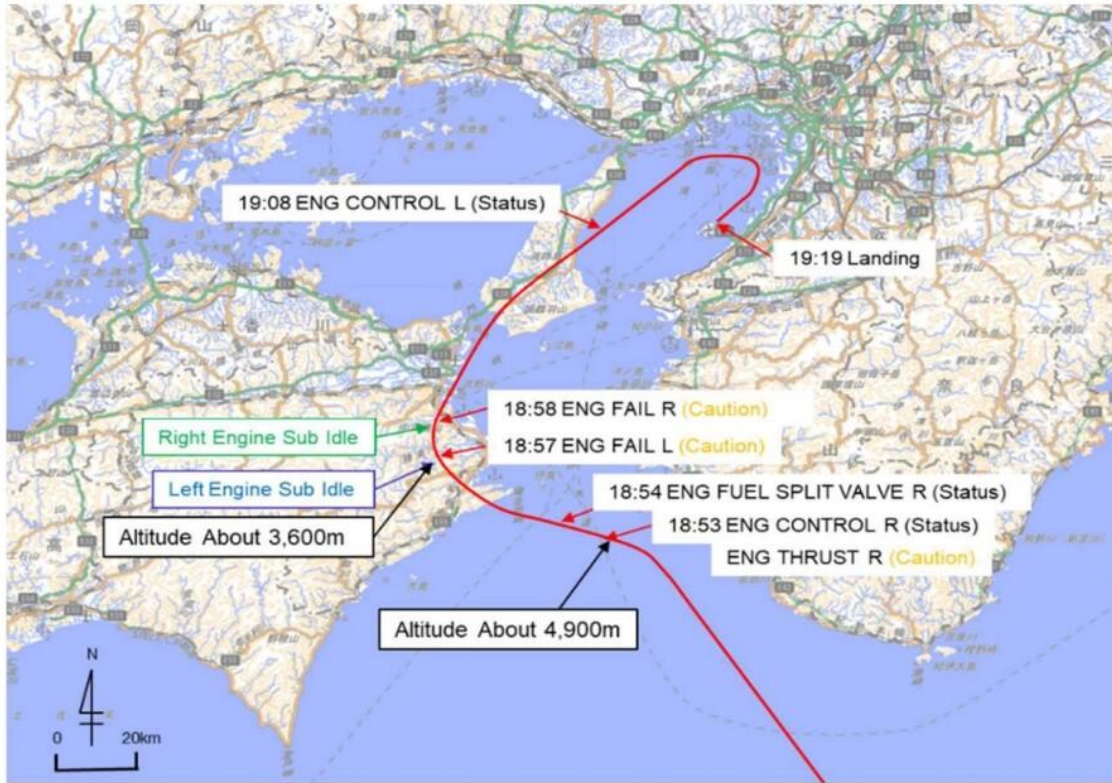
Figure 10. Jetstar Airways Boeing 787-8 VH-VKJ GENx-1B Engine Incident Approaching Kansai
