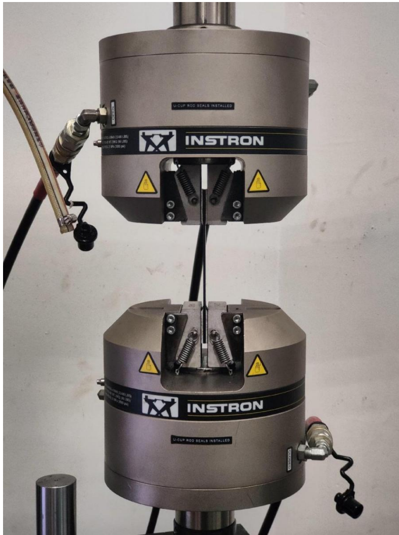
Fig. 2.10. Instron 8801 electro-hydraulic servo fatigue machine.
