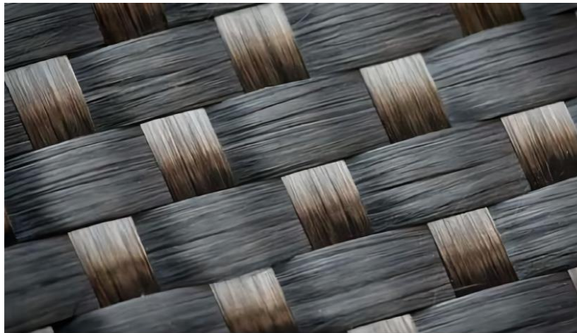
Fig. 2.1. Carbon fiber weave texture map.
