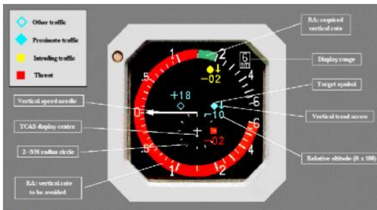
Figure 1.4. TCAS RA Display Implemented on an IVSI
