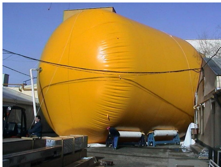
Figure: 4.8. Soft storage system with bridges
