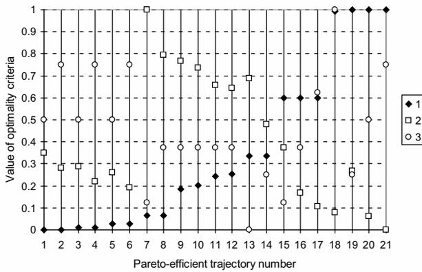
Fig. 2. Optimality criteria values: 1– regularity criterion  $c_1$ ; 2 – efficiency criterion  $c_2$ ; 3 – criterion of maneuvering complexity  $c_3$
