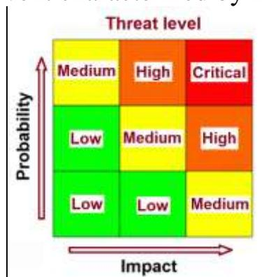
**Fig. 5 Impact of the accident vs. its probability.**
